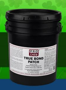
TRUE BOND PATCH is a ready-mix compound of finely graded mineral aggregate and specially prepared asphalt and additives for repairing holes and expansion joints in asphalt surfaces. It sticks to asphalt without a primer, even in cold, wet weather.
