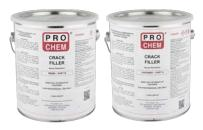
**Appearance** Clear liquid Odor Almost none Pot Life 15 min at 75°F Tack Free - 2-3 hours at 75°F, Light traffic **Dry Time** 8-12 hours, Full cure - 7 days 250 Sq Ft at 6 mils Coverage
