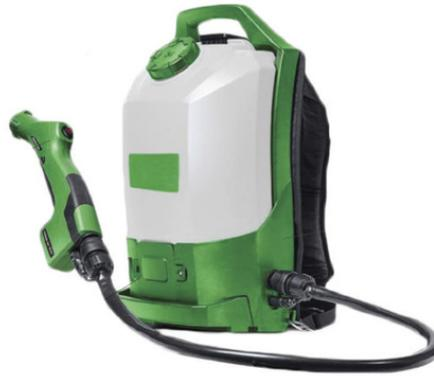
This ELECTROSTATIC SPRAYER provides many unique characteristics that cannot be found on other sprayers. It double charges the solution it is spraying. The product is charged when it enters the tank and again when it is sprayed. As the fully-charged droplets hit the surface, they create an even spread. When you spray something that has a negative or neutral charge, the product sprayed will not only
