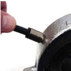
7. Insert the other end of the tubing in lube point fitting.
