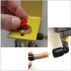
1. Remove plug from inlet and short shipping tubes from fittings.
