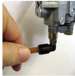
6. Cut tubing to the desired length. Insert into the distribution valve fittings.
