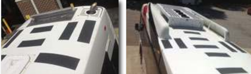
Use ANTI SKID TAPE for traction on the top of buses
